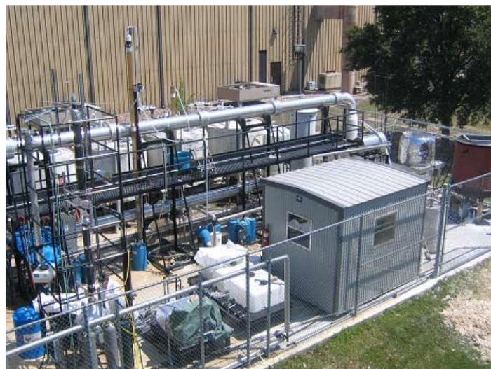
and butyric acids. The VFAs combine with calcium carbonate to form carboxylate salts, which are extracted from the pile with water.
